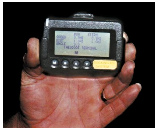
Mooring Line Monitoring Screen
